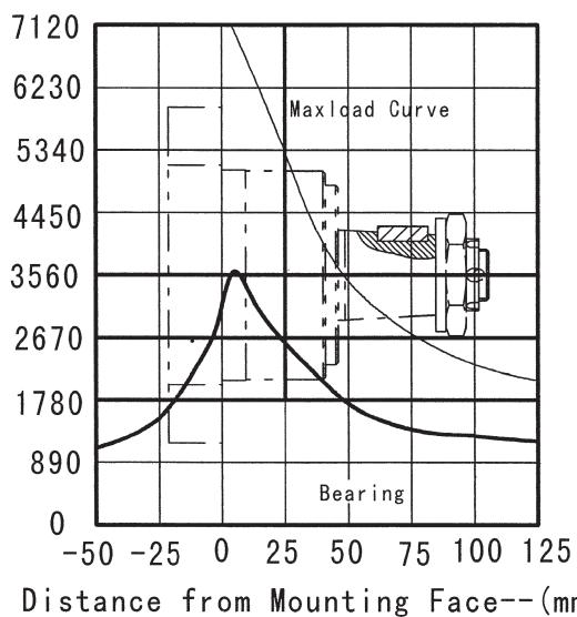
The bearing curve represents allowable bearing loads for an  $L_{10}$  bearing life at  $3 \times 10^6$  revolutions.
